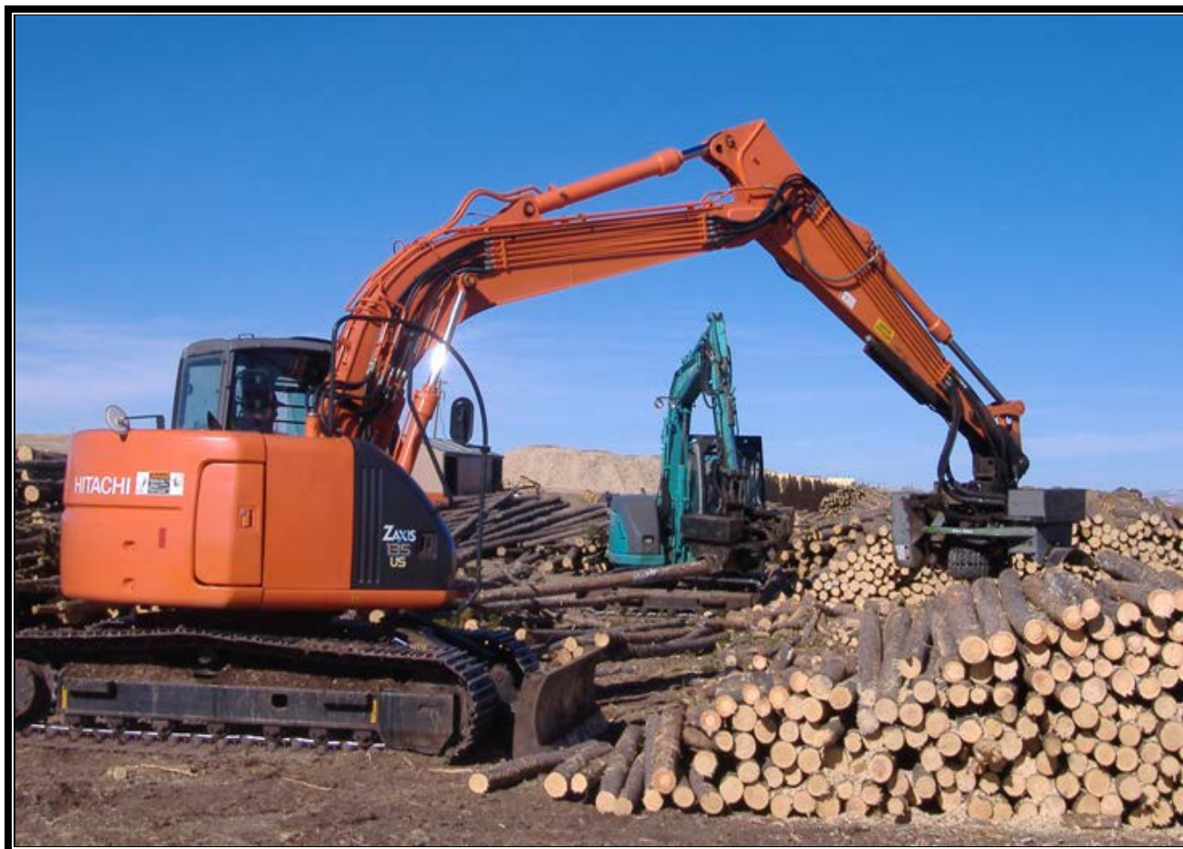
Figure 4.5 – Example of a Log Yard Processor (source Lodgepole Products, Inc.)
