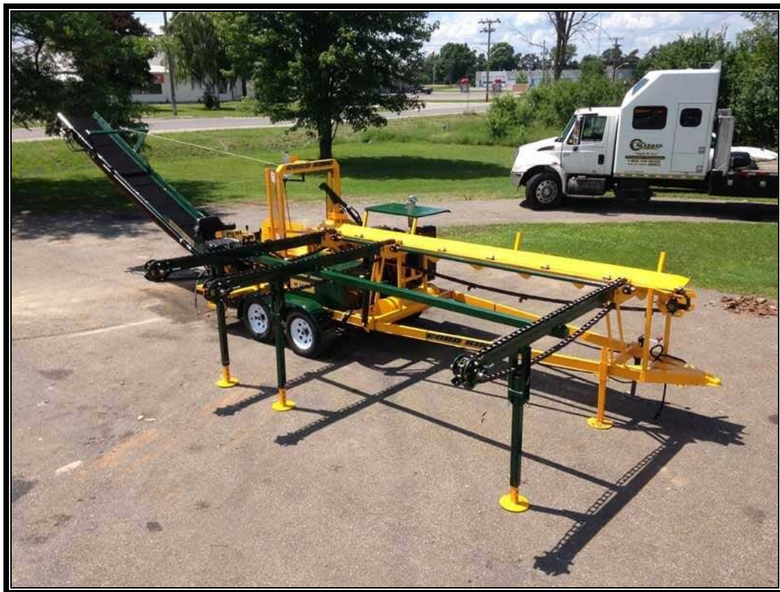
Figure 4.2 – Example of a Bar Saw Type Firewood Processor
