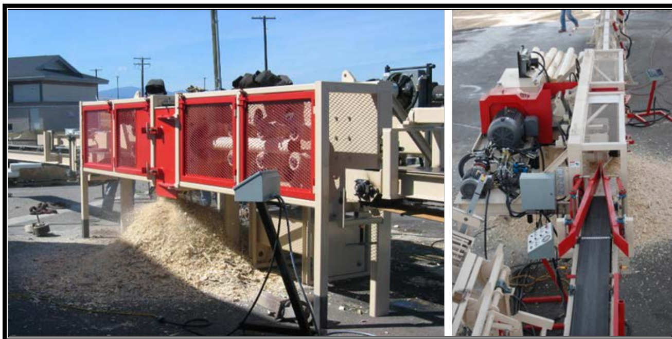
Figure 4.4 – Example of a Dowelling Machine (source Roundwood Systems )
