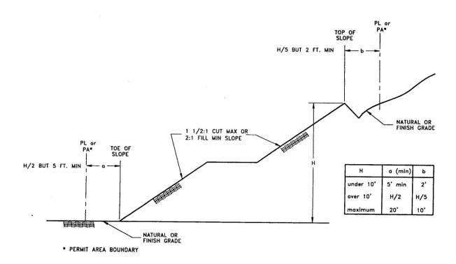
**12.20.290 Setbacks - Design standards.** Setbacks between graded slopes (cut or fill) and structures shall be provided. (See Detail #3.)
