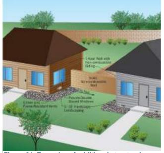
Figure 61. Examples of additional structural hardening and defensible space features where 30 feet of setback to the property line is not feasible (FEMA).
