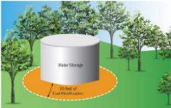
Figure 62. Providing appropriate vegetation clearance around critical water infrastructure and associated equipment is key for increasing wildfire resiliency.
